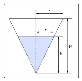
As we can see, the water in the tank actually forms a smaller cone/triangle (depending on which image we are looking at) with the same central angle as the tank itself. The radius of the "water" cone at any time is given by r and the height of the "water" cone at any time is given by h. The volume of water in the tank at any time t is given by,
