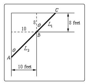
The largest pipe that can go around the turn will do so in the position shown above. One end
