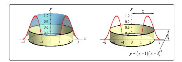
Doing this gives us a cylinder or shell in the object and we can easily find its surface area. The surface area of this cylinder is,
