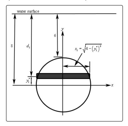
The depth below the water surface of each strip is,
