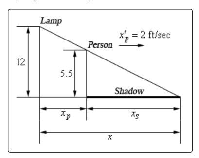
Here x is the distance of the tip of the shadow from the pole,  $x_p$  is the distance of the person from the pole and  $x_s$  is the length of the shadow. Also note that we converted the persons height over to 5.5 feet since all the other measurements are in feet.
